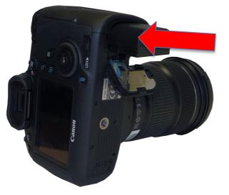
2. Insert the Media Card in the card slot of the camera. (The card should be inserted as shown in the photo)
